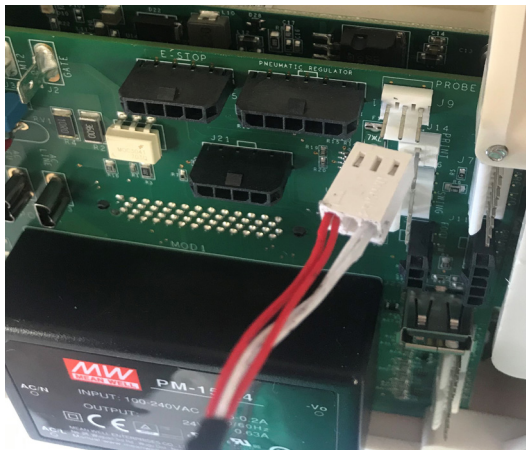
the 3-pin Temperature Probe Connector from the Controller depressing locking clip.
